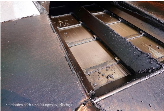
Scraper floor of asphalt pavers before and after treatment with Divinol Asphalt MP
